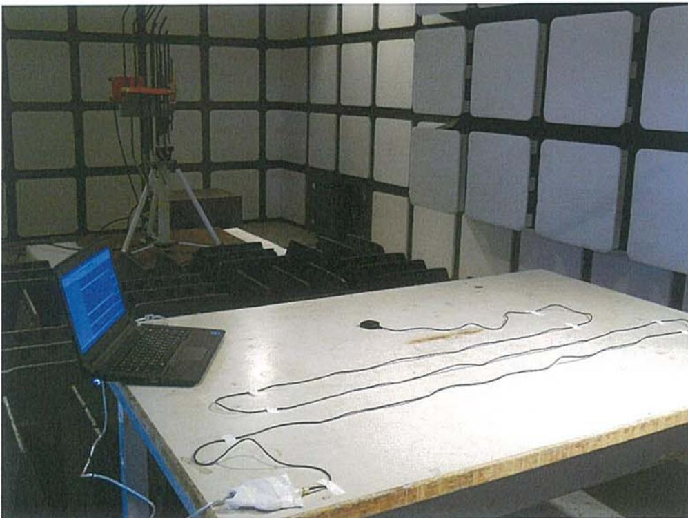
**4. EFT/Burst Immunity Test Setup Photo**
