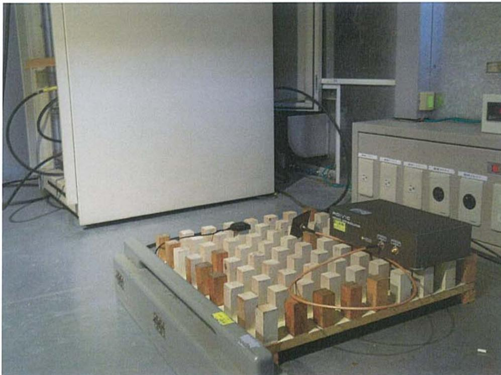
**6. Power Frequency Magnetic Field Immunity Test Setup Photo**
