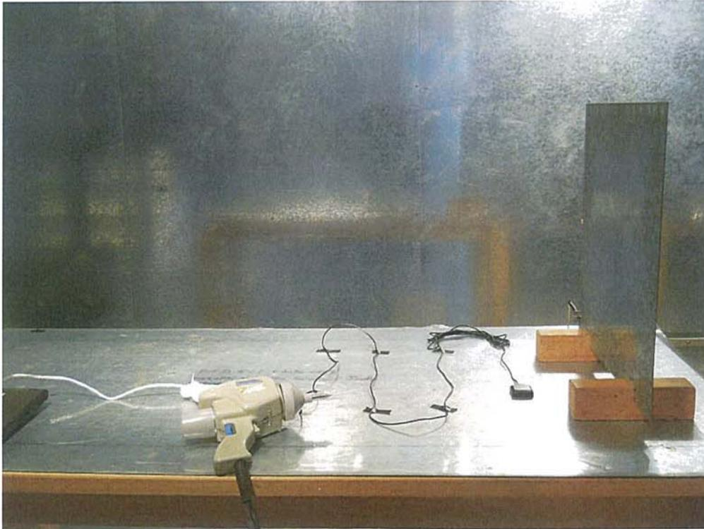
**3. RF Radiated Fields Immunity Test Setup Photo**
